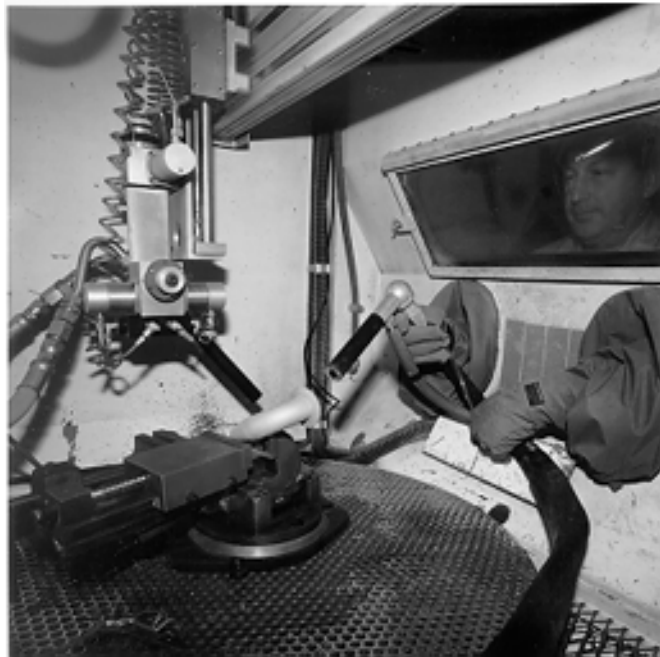
Figure 2 Inside Glove Box Where A Hand-Held Duck Gun Performs The Clean
