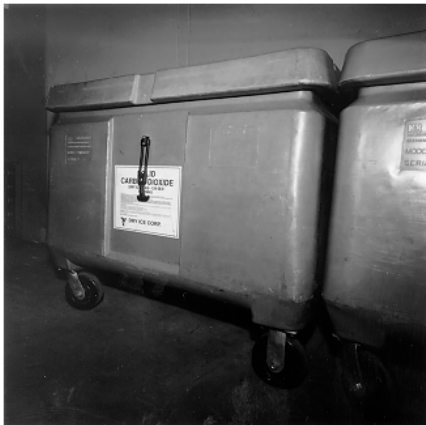
Figure 5 Storage Containers for Dry Ice
