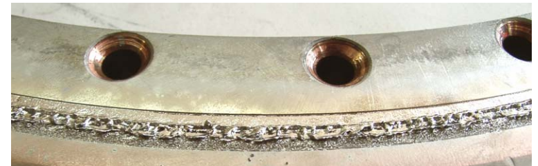
Tin surface after 6 millions pulses if system of tin surface regeneration is not used
