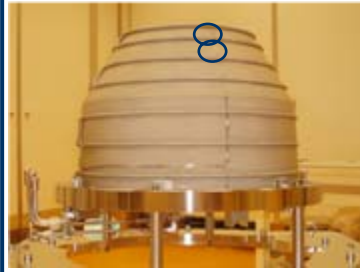
2. 20 thermocouples installed in strategic locations
