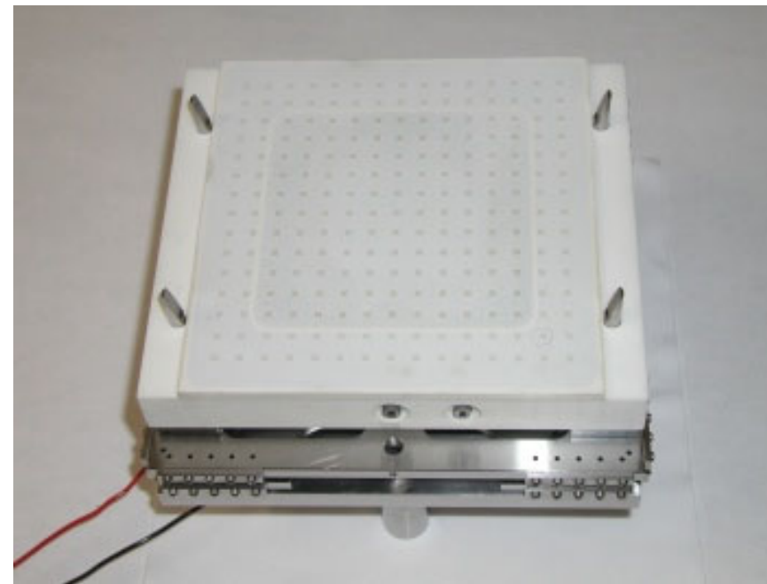
Chuck placed on the Lifter System
