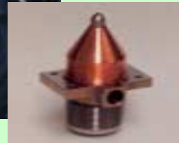
Comprehensive xenon jet test capability Measuring source angular distribution, size, shape, stability, repeatability and contamination
