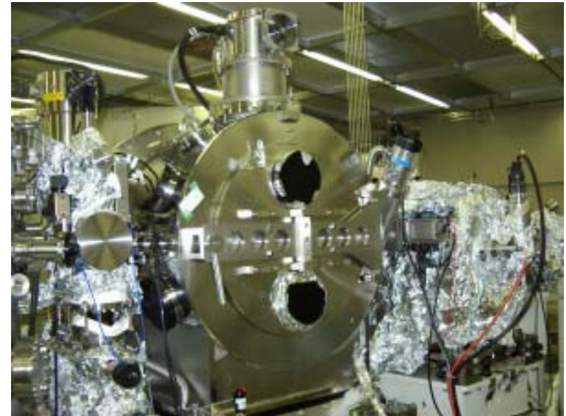
The EUV reflectometer at ASET Atsugi Site.
