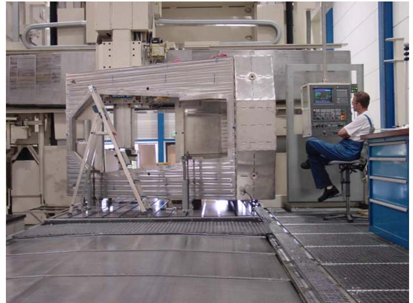
Baseframe Mainbody, during Coordinate Measurement Machine qualification.
