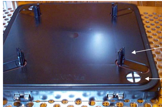
RSP Base Showing Plate Holder Posts "O" Ring and Filters
