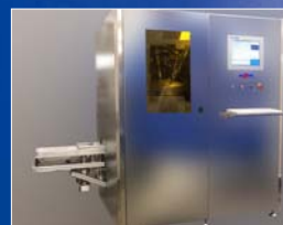
High-Throughput EUV-Reflectometer from AIXUV (20 - 40 s per 0.1x1 mm spot)
