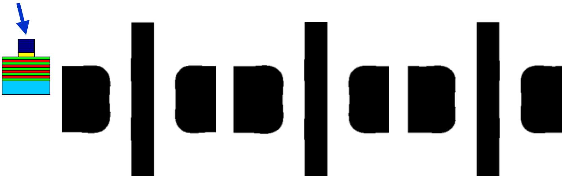
(a) Binary mask Ta 34nm/Cr 30nm NA: 0.25, \sigma : 0.80
