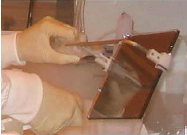
EUVL masks consist of a patterned absorber of EUV radiation placed on top of an ML reflector deposited on a robust and solid substrate.
